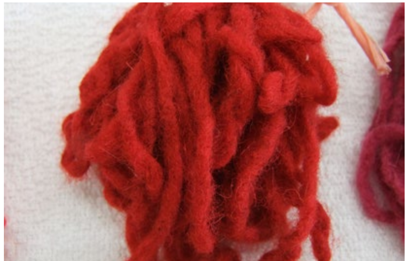
FIGURE 9. Wool without mordants dyed in a laboratory with cochineal in an acidic medium (Photograph: Sergio Franco Maass, 2017).
