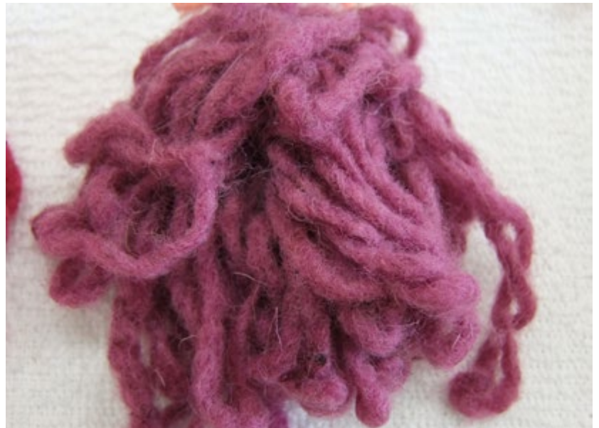
FIGURE 11. Wool processed with potassium dichromate mordant and dyed in a laboratory with cochineal in an acidic medium (Photograph: Sergio Franco Maass, 2017).
